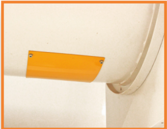
Emergency Unloading Gate
